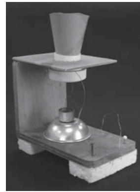
Figure 2. A student's recreation of Bell's liquid microphone—the world's first microphone.
