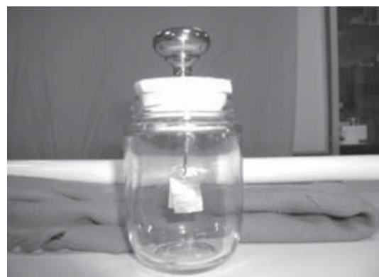
Figure 1. Photo of an electroscope used for demonstration purposes during the lecture made by the lecturer using simple, readily available materials such as aluminium foil, a paper clip, a glass bottle and brass door knob.
